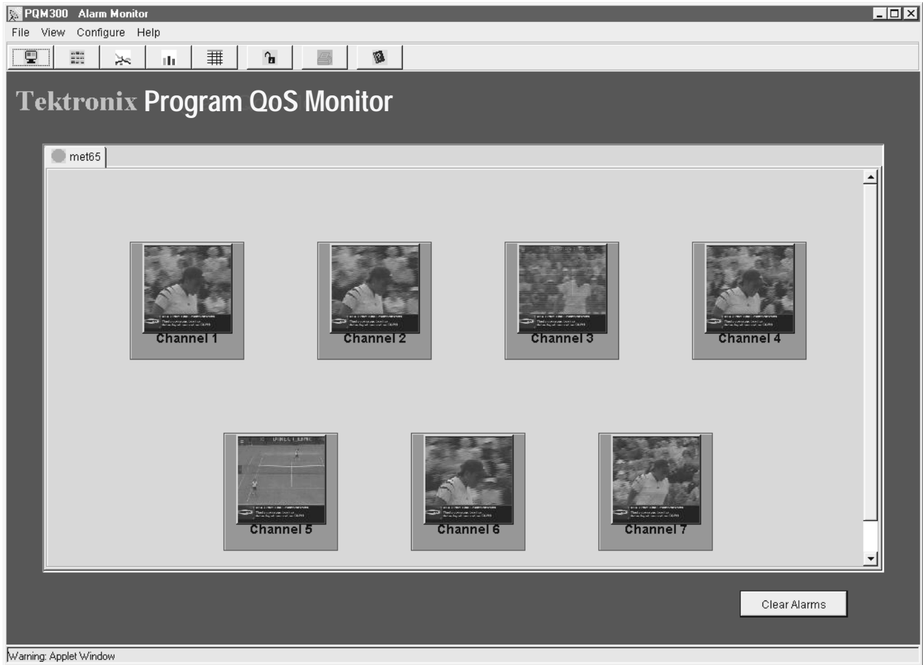
Figure 2-3: Alarm monitor by connection view
